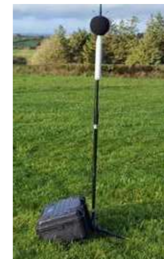
Typical noise monitor used to measure background noise levels during the design process
